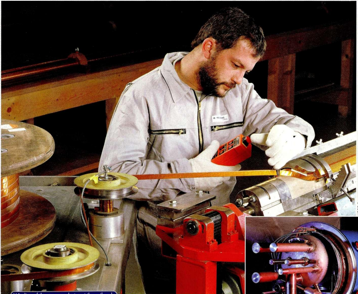
Winding of the superconductor at the coil end
